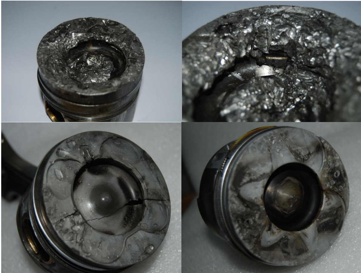
Fig. 2. Mechanical piston damage
