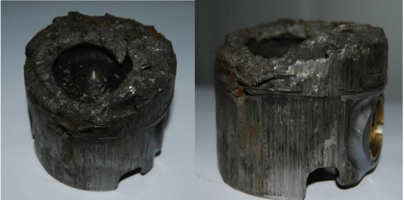
Fig. 3. Fusion of the piston head and the ring area
