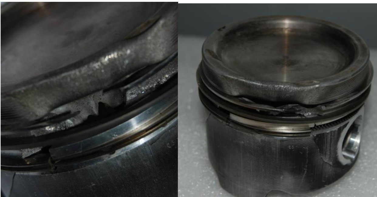
Fig. 1. Fusion of the piston head and the ring area
