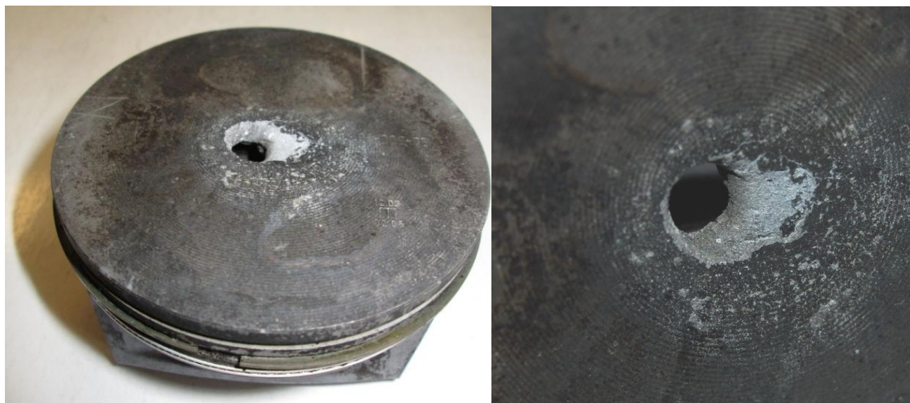
Fig. 6. A hole in the piston head in a spark-ignition engine is caused by a premature ignition or a hot-bulb ignition
